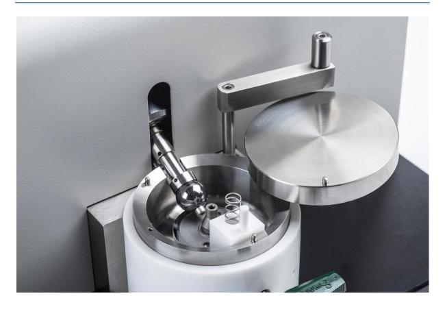
PTFE assembly that controls the flow of grease onto the disk while testing on the MTM.
