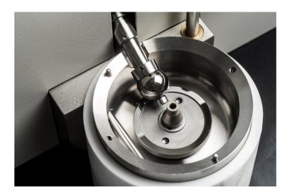
A PDMS ball and a PDMS disc were used as the test samples. These have a hardness of 50 duro.
