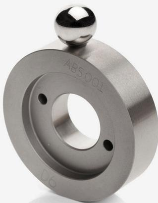
▲ ABS Test Cylinder and Ball Specimen
