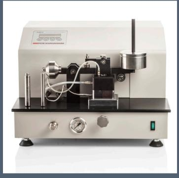
A fully automatic laboratory instrument for evaluating the scuffing load resistance of diesel (middle distillate) fuel according to ASTM D6078.
