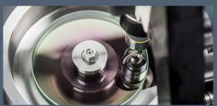
A fully automated, benchtop instrument, measuring lubricant film thickness down to 1nm in the elastohydrodynamic (EHD) lubricating regime.
