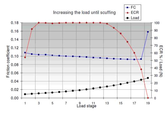
MTM2 results obtained running a scuffing test procedure
