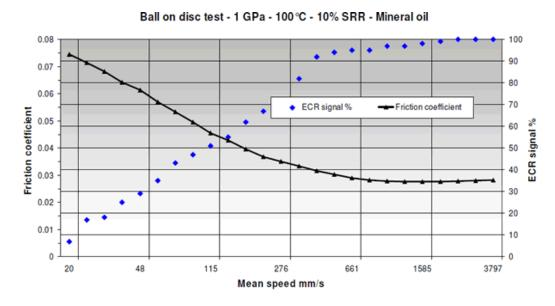
MTM2 result for a 'Stribeck' type of test using ECR set up
