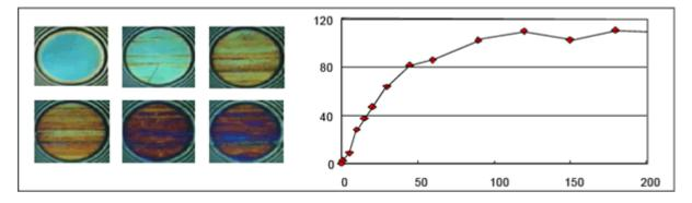
Figure 5: Images (from top left to right) from 0, 5, 20, 30, 90 and 120 minutes running of a fully formulated oil with ZDDP and resulting graph showing ZDDP reaction film thickness (in nm) against time
