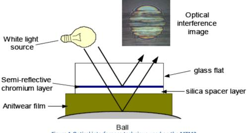
Figure 1:Optical interference technique used on the MTM2
