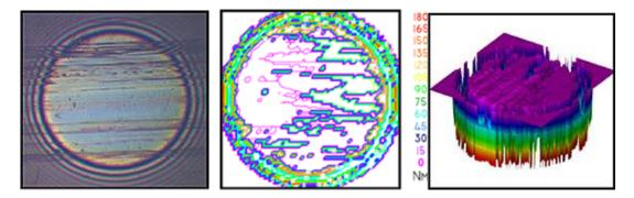
Figure 4:Image taken during test, 2D Contour Map, 3D Surface Map
