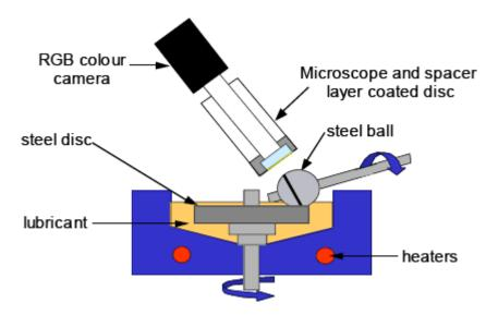
Figure 2: Step 1 – The test ball is run against a steel disc for a pre-defined time
