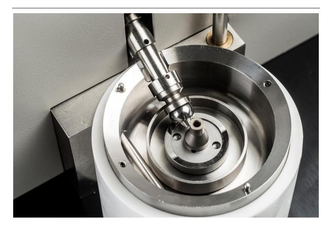
Assembly that allows lubricant sample size to be reduced to 4ml and foreign bodies to be simply introduced to the test sample.
