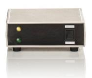
The MTM oil cooler can be controlled by the MTM software to turn on after tests and cool the test cell down to a user defined temperature. This allows faster turnaround between successive tests at high temperature.
