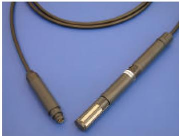
The ambient temperature and humidity is recorded using the HFRR integrated humidity probe. A humidity checker is available from PCS.
