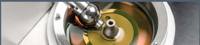
A ball-on-disc instrument for measuring the frictional properties of lubricated and unlubricated contacts under a wide range of rolling and sliding conditions.
