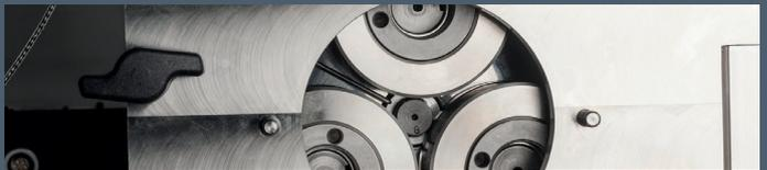
Triple disc machine for researching rolling contact fatigue (RCF) failure mechanisms in the form of micro and macro pitting under lubricated and unlubricated conditions.
