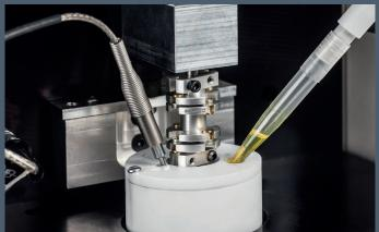
A high shear viscometer measuring viscosity up to 10 million reciprocal seconds.
