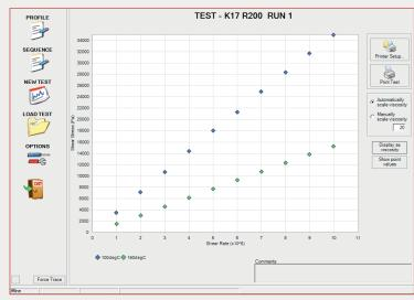
Viscosity against shear rate for a non-newtonian fluid
