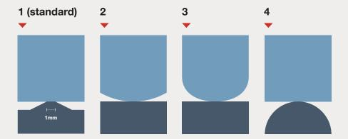
MPR pressures using various specimen geometries
