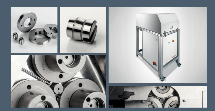
Triple disc machine for researching rolling contact fatigue (RCF) failure mechanisms in the form of micro and macro pitting under lubricated and unlubricated conditions.
